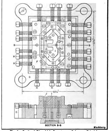
Fig. 6. Sectional Die which Operates on Sub-press Principle
